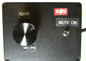
All sound goes through the **volume knob**, which is an active attenuator and has a MUTE switch.
